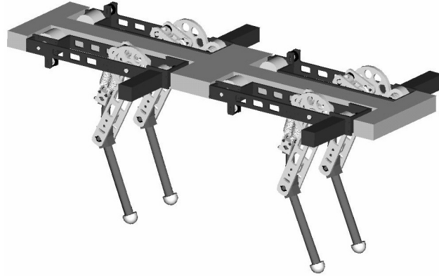
Figure 7.3: Solid model of the quadruped design with legs matching the existing prototype leg.
