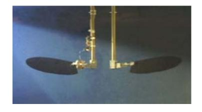
Dickinson et al. built "robofly" - large robotic wings that flap slowly in a vat of mineral oil
