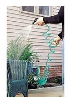
Water nozzle reduces A<sub>out</sub>, so u<sub>out</sub> increases
